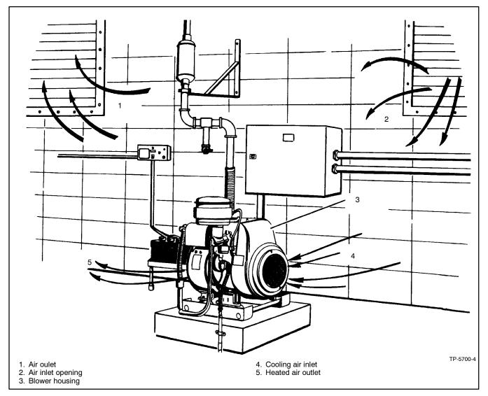
Figure 4-5 Standard Forced-Air Cooling System
